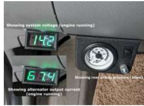
Volt/Ampmeter and Aigbag pressure and controls. (double picture of meter showing alternator voltage and current Output. Switches between them every 5 seconds)
