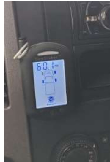
This is the TireTracker TPMS located next to the radio.
