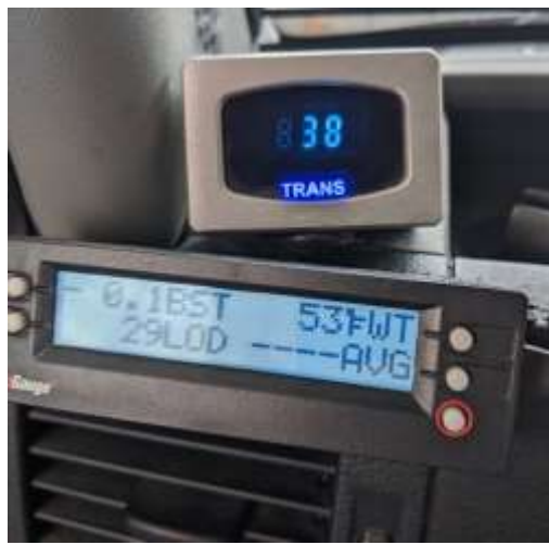
Digital Temp Gauge and Scangauge II, set for Boost, Engine temp, Load, and Average MPG
