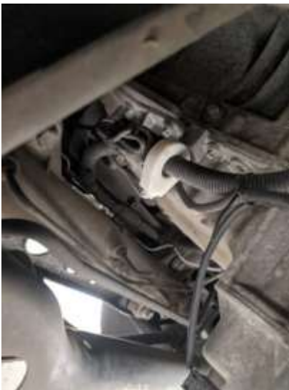
This is where the Hall Effect transformer is located on the output harness from the alternator. I only want to see the alt. output, and the only other draw is for the aux. fan which has it's own connection.
