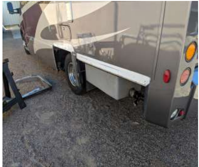
Rear panel and wheel skirt removed. Notice that there is NO FRAME or other support here.
