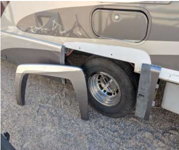
I had to saw cut a section of the panel so I could get the wheel trim back in place.
